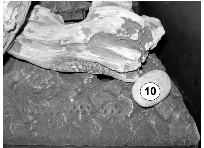
Figure 7.35. Engage blocks in the underside of Left Lower Rock #4 with the adjacent pockets on the burner base by Log #4.
