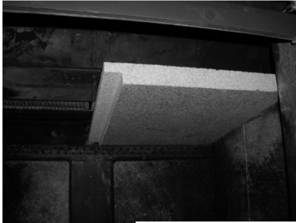
Figure 19b – Removing / Replacing the Baffle
