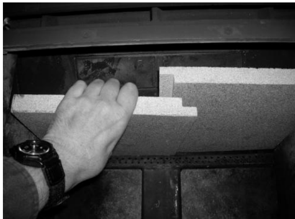
Figure 19a – Removing / Replacing the Baffle
